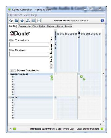
also quickly and easily backup, restore, move, and reuse Dante network configurations using Presets, and edit Dante routing configurations offline.
